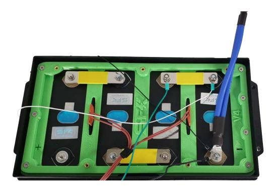
Now you will add your series terminals and BMS balancing/monitoring wires as well as the active balancer wires (NOTE the initial negative post; and the final positive post are shared between both the active balancer & BMS, all other posts may be separate for each cell). Place the BMS ring terminal directly over the main lug and then the active balancer ring on top of it.
