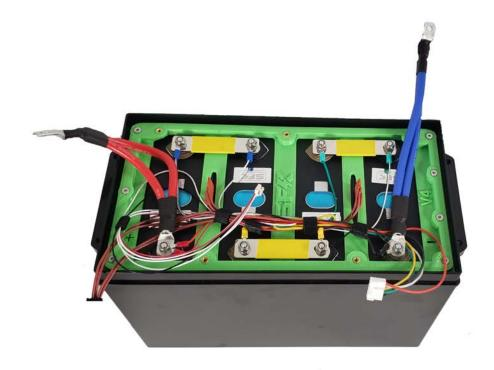
Your cells should come with the bus bars and terminal studs or welded terminals. Tidy up your install using electrical tape, zip ties, or velcro strips. Setup the wiring schematic as follows:
