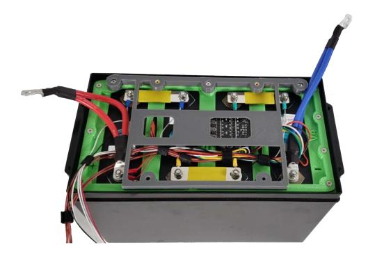
Once installed the active balancer should have a small amber light appear letting you know it is working, we now move on to the BMS mounting plate.
