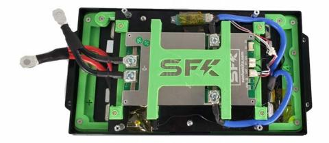
Install the wires as shown and route the wires to best suit your needs, you can use the included wire keeps to assist in cable management. **NOTE: do not connect the BMS balancer wire until you have installed the lid & lugs.**
