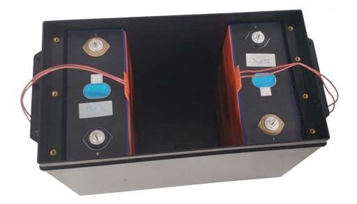
Test fit the cells to get an idea of the installation; you will now need to prepare the cells with shims. For this you have 2 options:
