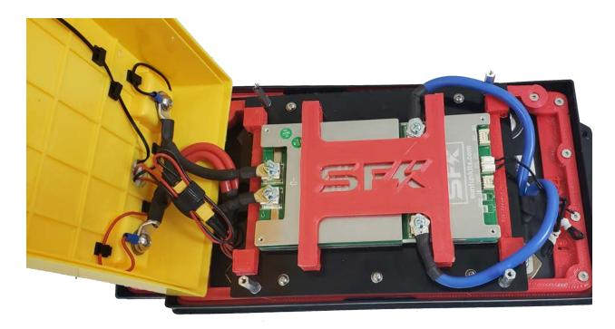
Connect the heating pads to the thermal switch's XT30 plug, this is a Y-PLUG and will be able to provide power to both heating pads. Once connected you can route the harness below the BMS plate to tuck it away and provide ample room to attach the wires to the lid.
