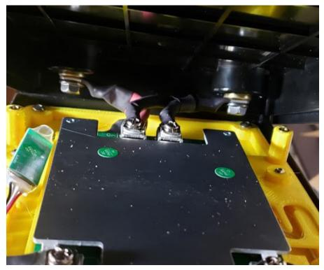
Once this lid is removed you can investigate the bolts to ensure a tight slop free fit.
