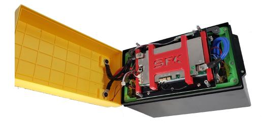
We only recommend opening the lid of your battery with hand tools and not with powered screwdrivers or impact drivers. Only use insulated tools when working with the battery with its lid open.
