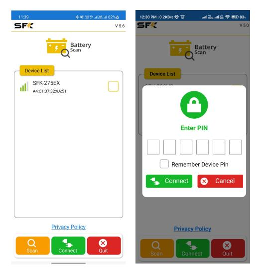
After you have downloaded the app, you will need to enable location services to allow a connection to your SKF-275EX battery. Once enabled you can scan for available devices and connect to the battery you wish. With version 4.X and higher; the SFK BMS app supports up to 4 simultaneous device connections, this is explained on page: 39.
