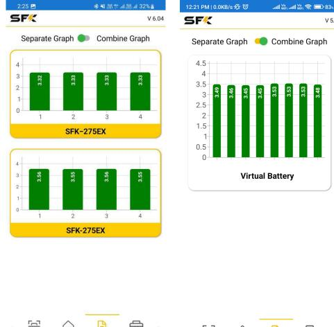
When connected to Multi-View you will notice various options that differ from the single view. Here you can analyze information that represents all of your connected batteries as a single bank. The details tab will display information for your cell voltages per pack, or you can view them together in a single large graph. This is useful to ensure all of your cells are balanced and are working properly as well as able to hold voltage under load.
