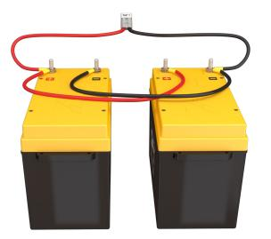
In all parallel setups, you must ensure your cables are of equal length, we recommend using 2 AWG or lower gauge for best performance.
