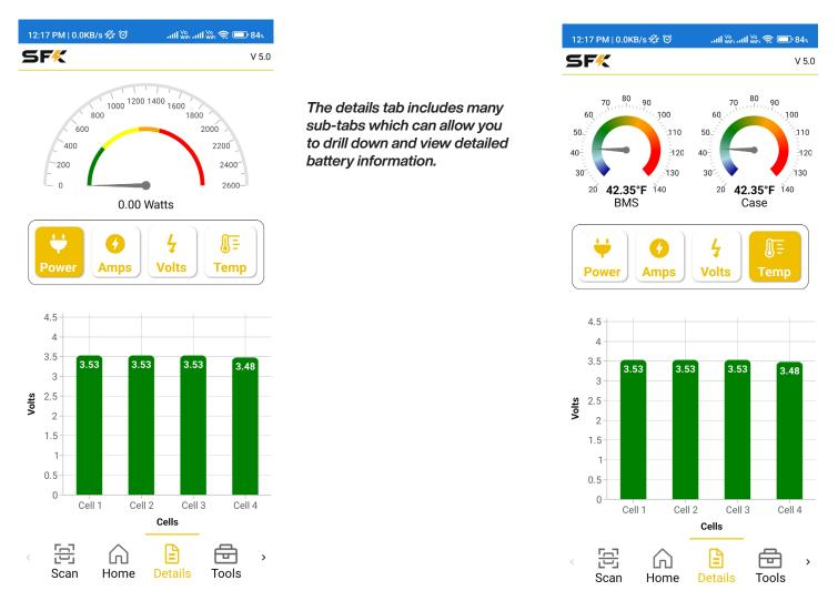
The details tab provides additional information for your battery, this can be useful in finding out issues you may be experiencing such as HVC or LVC (high/low voltage cut-off). If you are finding your cells are being stressed under loads you can use the information to make changes to the load accordingly. NOTE: The SFK-275EX has 3 temperature probes which includes 1 BMS probe and 2 case probes, you can switch between the case probe temps by clicking the case temp gauge to switch between them.
