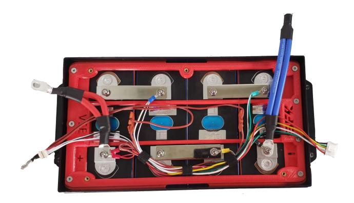
Note: CAUTION!!! In many prismatic cells the positive terminal is colored black and the negative terminal is colored brown! Please double check your cells with a volt/multimeter before continuing. THE BLUE WIRE SHOULD NOT TOUCH THE POSITIVE TERMINAL OF THE FIRST CELL OR IT WILL ARC AND DESTROY THE CELL.
