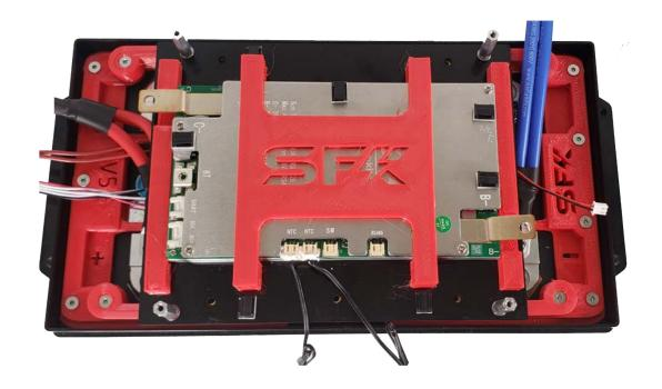
You can place some of the stick on wire keeps as needed, this will assist in securing wires used by the Gen 2 I/O switch. The SFK-200 BMS includes 2 external temp probes, these can be mounted in the positions of your choice, use the included stick-on wire keeps as well as Kapton tape to mount them into position.
