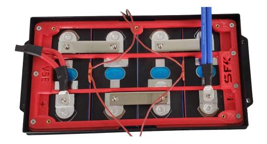
Now you will add your series terminals and BMS balancing/monitoring wires as well as the active balancer wires (NOTE the initial negative post; and the final positive post are shared between both the active balancer & BMS, all other posts may be separate for each cell).
