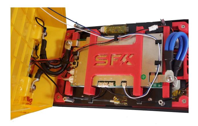
Once done, review your wire installation and make sure when the lid is closed it is **NOT PINCHING** any wires **AND ONLY WHEN ALL THIS IS DONE**, **SHOULD YOU INSERT THE BMS BALANCING WIRES into the BMS** to complete the inside install.
