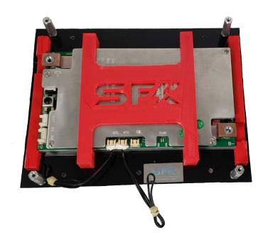
Note: Before beginning this step it is EXTREMELY IMPORTANT that you clean and wipe down all of your bus bars, washers, terminals and battery post with 90% isopropyl alcohol. Dirty terminals and connections will result in improper readings and poor results.
