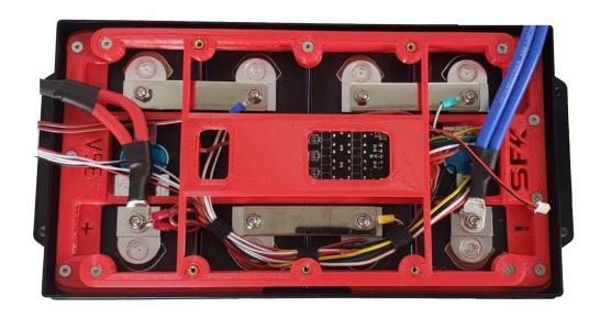
Secure the riser plate using the 4 countersunk M4x20mm screws on the sides. We recommend only using hand tools for this process.
