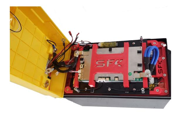
Mount the black main lug to the BMS using the included M6 bolts and hex nuts. Secure the blue wire to the bms using the same method. A M10 wrench is recommended to keep the hex nut in place.
