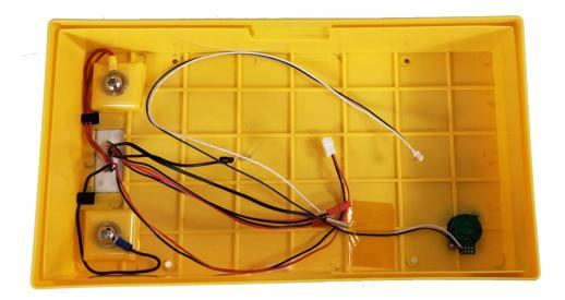
During the injection molding process some residual abs material may have gotten deposited onto the main brass conductor rings, these need to be cleaned. Using 300-400 grit sandpaper, gently scrub the conductor ring until all traces of residual abs plastic are removed.
