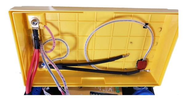
Mount the black main lugs to the BMS using the included dual M6 bolts note: the wires have a slight u-bend to them as this provides sufficient slack for you to open/close the lid as needed.
