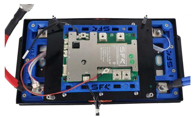
You can place some of the stick on wire keeps as needed, this will assist in securing wires used by the Gen 2 I/O switch. The SFK-8S-100 BMS includes 2 external temp probes, these can be mounted in the positions of your choice, use the included stick-on wire keeps as well as Kapton tape to mount them into position. Also included is a high temp thermal disconnect that may be mounted near the 8th cell.
