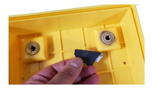
Once cleaned, use isopropyl alcohol to wipe clean and then begin to attach the main BMS and cell wires. You will attach the main negative (black wire) harness to the lid and then begin attaching the remaining wires to the battery.
