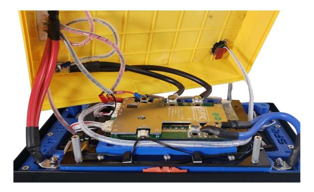
Attach the Bluetooth switch control using the JST connectors, then tuck the remaining wire underneath the BMS plate.
