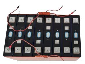
We are using dual heating pads in a 24v configuration and these are attached to the sides of the cells to provide for adequate battery heating.
