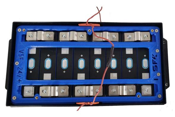
Begin by placing your bus bars in the orientation shown below, you DO NOT need to put a washer on top of the bus bars with the combination harness as it is using a large lug connector which acts as a washer, but you may put a washer on the posts that do not have a balance lead attached to it.
