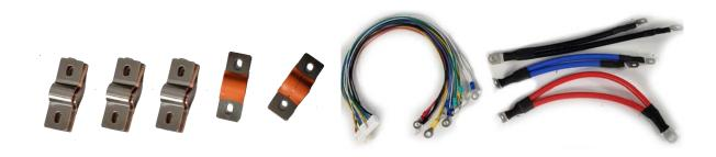
The V5 24 volt kit uses flexible busbars, these include a small heat shrink wrapping on them and needs to be removed to ensure proper contact with the larger terminals on the REPT 150 cells, use a utility knife to cut the heat shrink and remove it. V5 kits have pre-cut and crimped bms/active balancer wires as well as the main power leads to connect the cells to the BMS.
