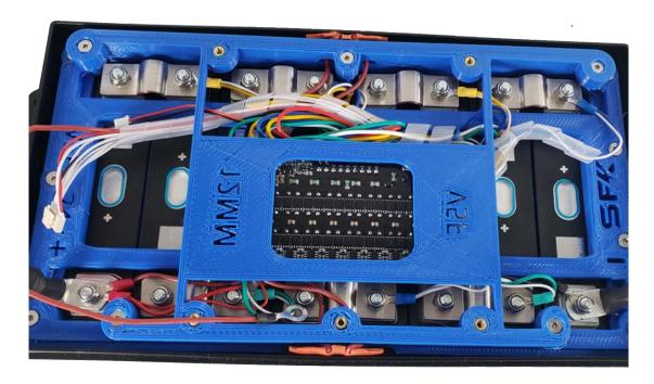
After this process we will now install the BMS plate. You will use 5 of the M4x16mm button head screws with a washer to secure the plate to the riser. With version 5 all bolts are now exactly the same.
