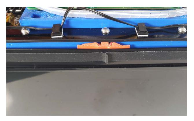
There should be sufficient length to cover the entire perimeter of the case, you do not need to stretch the rubber, but keep a firm grip to prevent slack while installing. Once done use a utility knife to remove any excess for a flush fit.
