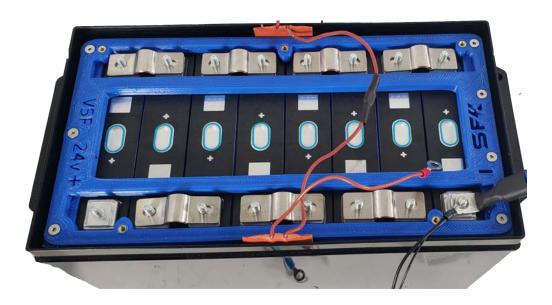
Now you will add your series terminals and BMS balancing/monitoring wires as well as the active balancer wires (NOTE the initial negative post; and the final positive post are shared between both the active balancer & BMS, all other posts may be separate for each cell). Secure using the included M6 Nylon insert nuts and tighten to 4-6 N/M.
