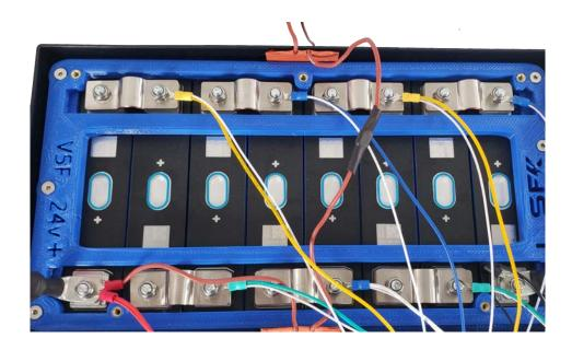
NOTE: The main power wires have a 90 degree bent lug, these attach to the cell.
