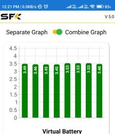
When connected to Multi-View you will notice various options that differ from the single view. Here you can analyze information that represents all of your connected batteries as a single bank. The details tab will display information for your cell voltages per pack, or you can view them together in a single large graph. This is useful to ensure all of your cells are balanced and are working properly as well as able to hold voltage under load.
