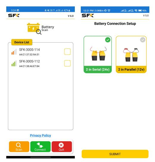
Once you have selected the batteries to connect to (maximum of 4), you can then inform the app on how you have them connected (e.g. in parallel, series, or parallel & series). This will then display information to you regarding the voltage levels, amps, and approximate state of charge of the batteries as a combined bank.
