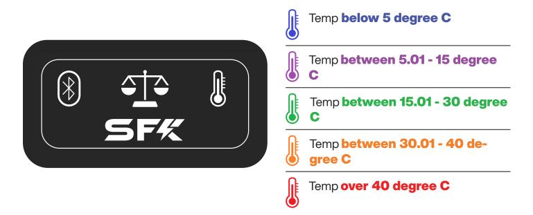
**Bluetooth:** Bluetooth functionality can be enabled by pressing the Bluetooth icon for 1 second and it will illuminate the Bluetooth icon. Pressing the button again will disable Bluetooth connectivity. **NOTE:** The monitoring app will not work unless Bluetooth is enabled.
