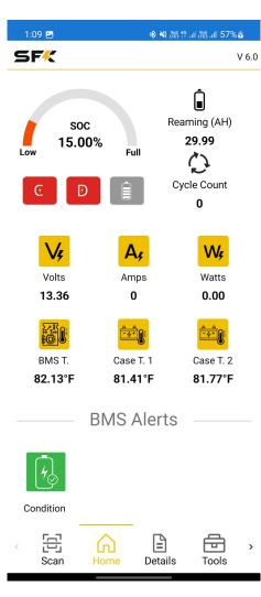
After downloading and connecting to your battery you can view information in 5 tabs. The Main tab will display general battery information like the state of charge of the battery, the temperature, remaining capacity, as well as the current and watt output.
