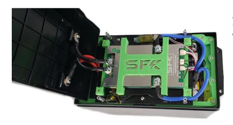
Only use insulated tools when working with the battery with its lid open.
