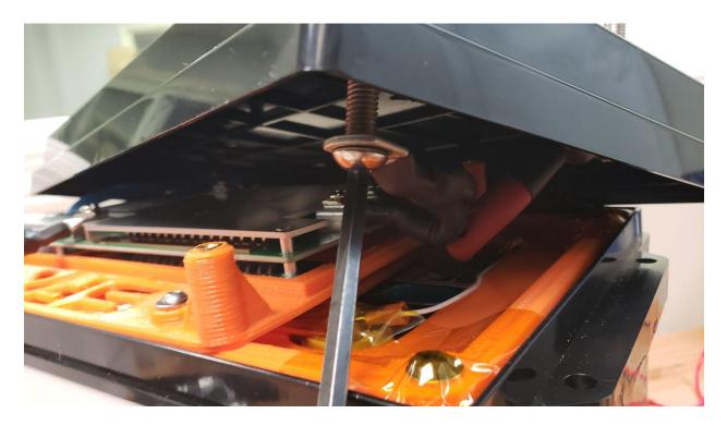
Using your hex driver, secure the bolt to the terminal, make sure you have the wires correctly oriented and that they are inserted into the correct terminal (red wire to the positive terminal and black wire to the negative)
