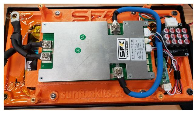
Secure components such as the Bluetooth dongle or supplementary balancer using double sided sticky tape. Also use Velcro strap to tidy up any loose wires. Use thread locker to secure the terminals to the BMS.
