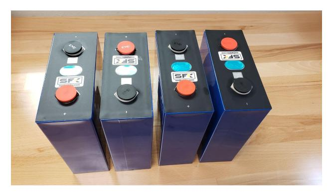
Before you can begin organizing your battery pack, you will need to perform a TOP BALANCE of your battery cells. This process requires you to charge your cells in parallel, meaning you will join the positive terminal of all your cells into a single circuit and your negative terminals into a single circuit.
