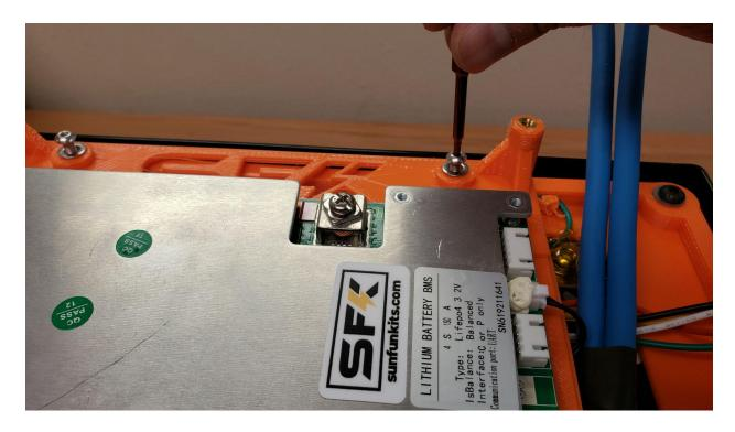
DO NOT USE POWER TOOLS TO ATTACH YOUR TOP PLATE, only use hand tools and tighten gently.
