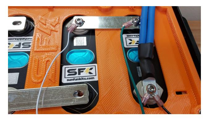
Sun Fun Kits include 6mm bolts that are 8mm in length; these will fit the drilled EVE 280N cells properly and will ensure a proper fit. Our BMS also includes correct sized terminals that fit 6mm threads/blots properly.
