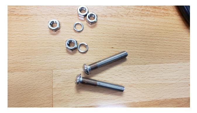
Prepare the m8 bolts with thread locker compound on the portion closest to the terminal head.
