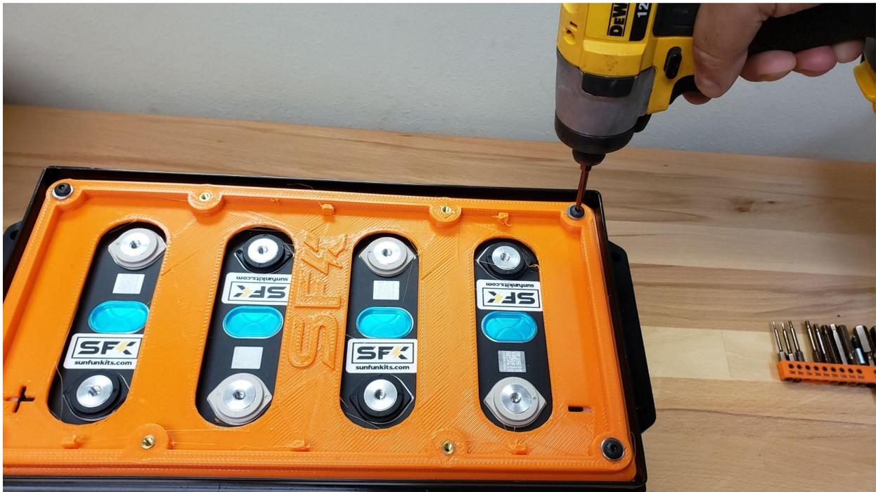
Install the bottom bracket with the M5 bolts and washers, you can use power tools to assist in this step.
