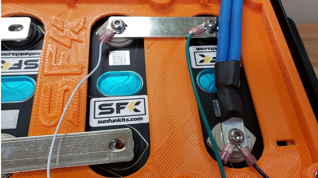
Sun Fun Kits include 6mm bolts that are 8mm in length; these will fit the drilled EVE 280N cells properly and will ensure a proper fit. Our BMS also includes correct sized terminals that fit 6mm threads/blots properly.
