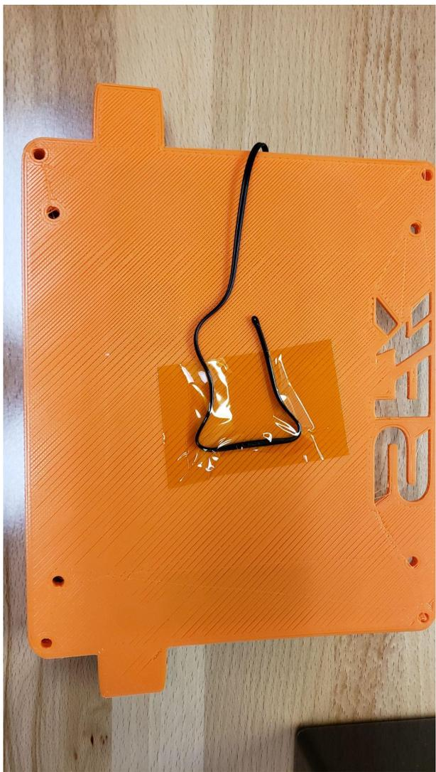
The SFK 150 4s BMS includes an NTP probe, this can be mounted on the underside of your top plate, or directly to any of the cells in the battery.
