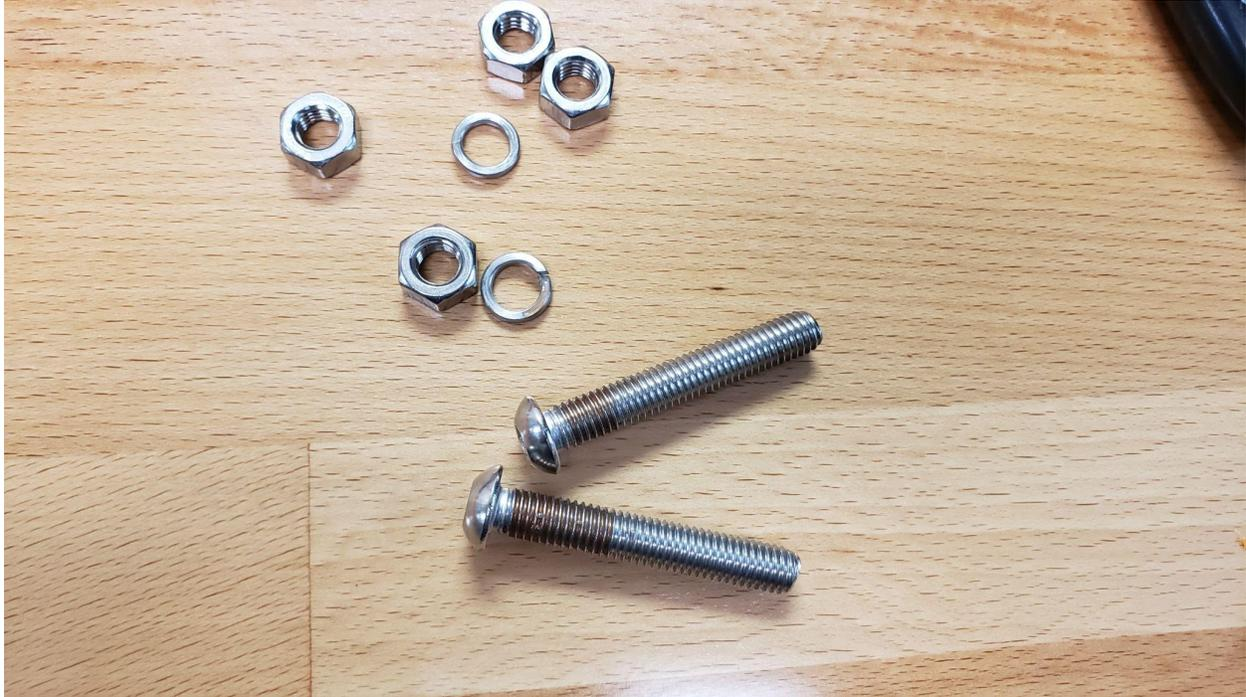
Prepare the m8 bolts with thread locker compound on the portion closest to the terminal head.
