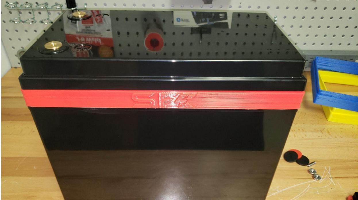
This shows how the v2 kits look from the outside, the lid and bottom are the same as the v1, but the spacer in the middle is unique to the v2 kit.
