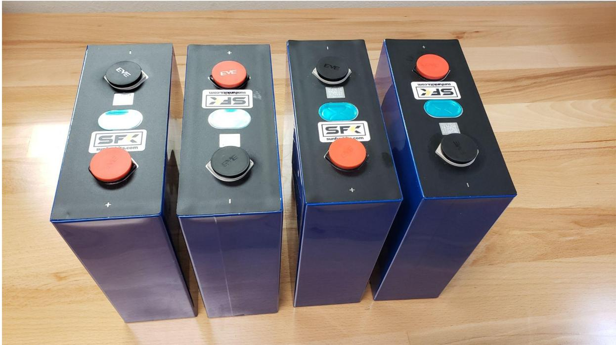
Before you can begin organizing your battery pack, you will need to perform a TOP BALANCE of your battery cells. This process requires you to charge your cells in parallel, meaning you will join the positive terminal of all your cells into a single circuit and your negative terminals into a single circuit.
