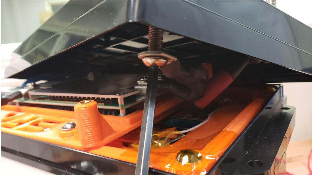
Using your hex driver, secure the bolt to the terminal, **make sure you have the wires correctly oriented and that they are inserted into the correct terminal (red wire to the positive terminal and black wire to the negative)**
