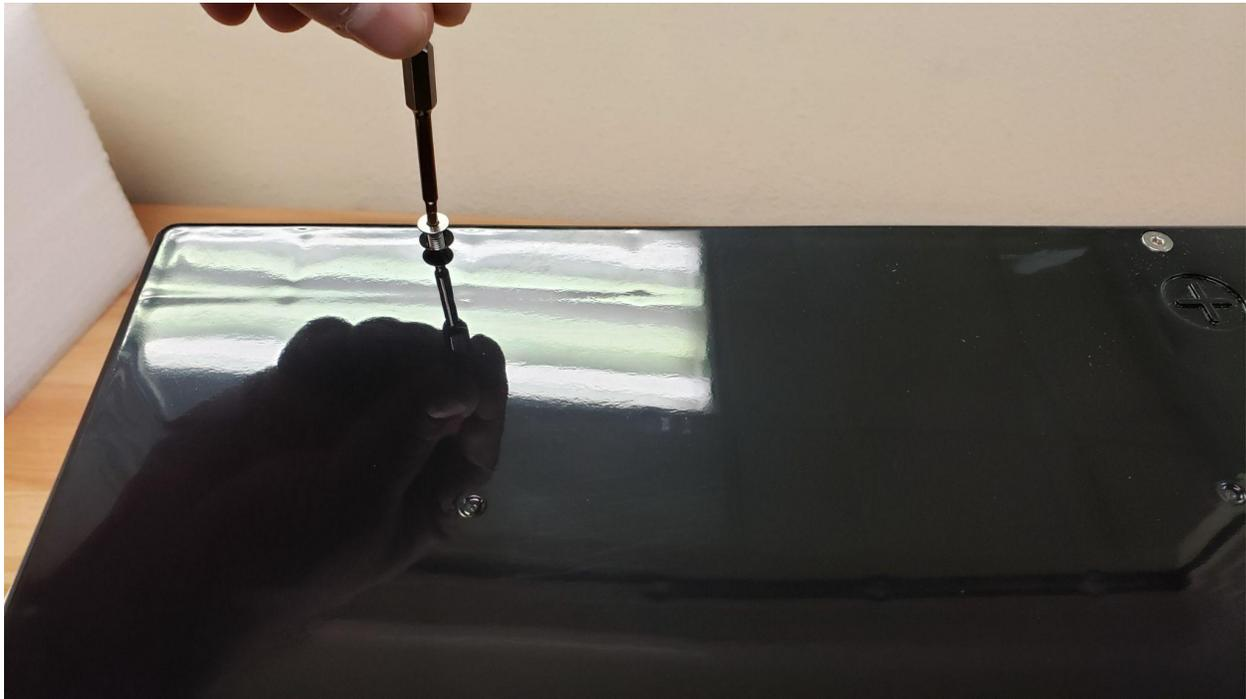
**NOTE:** If you prefer to increase water resistance you can add silicone sealant to the ridge of the lid before installing it, this will add a perimeter shield to assist in water/moisture intrusion while still keeping the lid removable. We do not recommend permanent glue or sealant in our kits.
