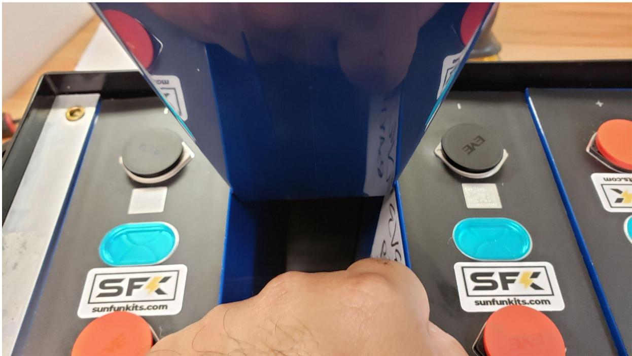
**Note:** you may find some resistance installing your cells, this is because the EPO foam exerts pressure on the cells to keep them in place. We recommend adding the left most and right most cells first and then adding the remaining 2 inner cells in the end.
