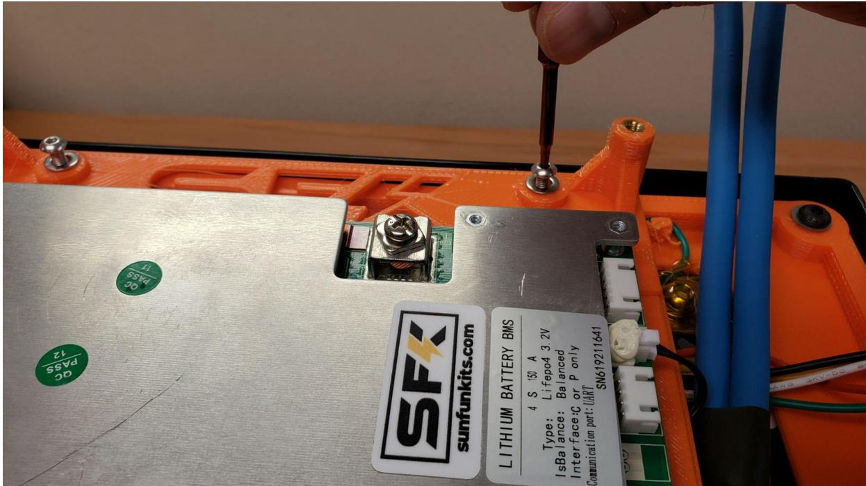
**DO NOT USE POWER TOOLS TO ATTACH YOUR TOP PLATE, only use hand tools and tighten gently.**
