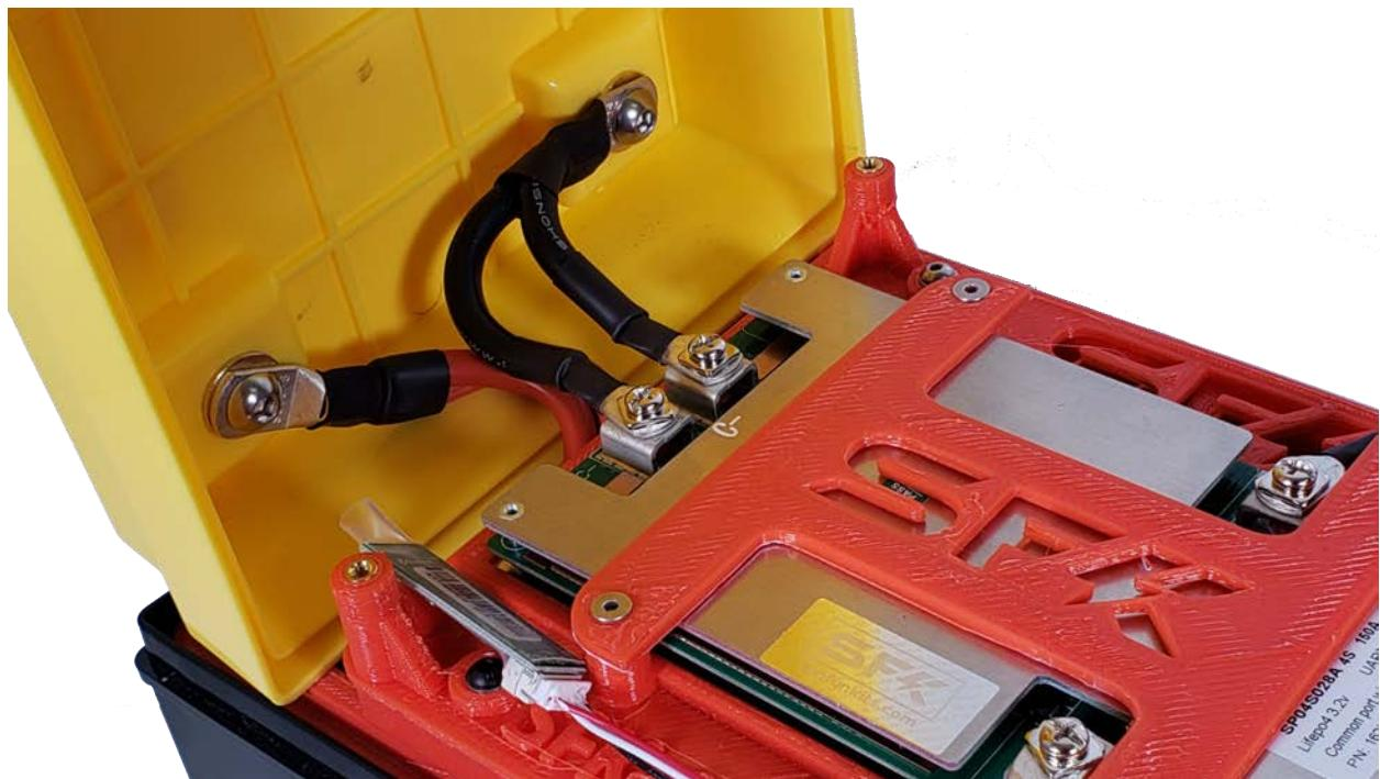
**ENSURE A TIGHT FIT!** You must make sure the bolt is making proper and solid contact to the brass insert, a loose contact will generate heat and can lead to battery failure. Ensure at least 10-15 NM torque setting (appx 140 inch/lbs).
