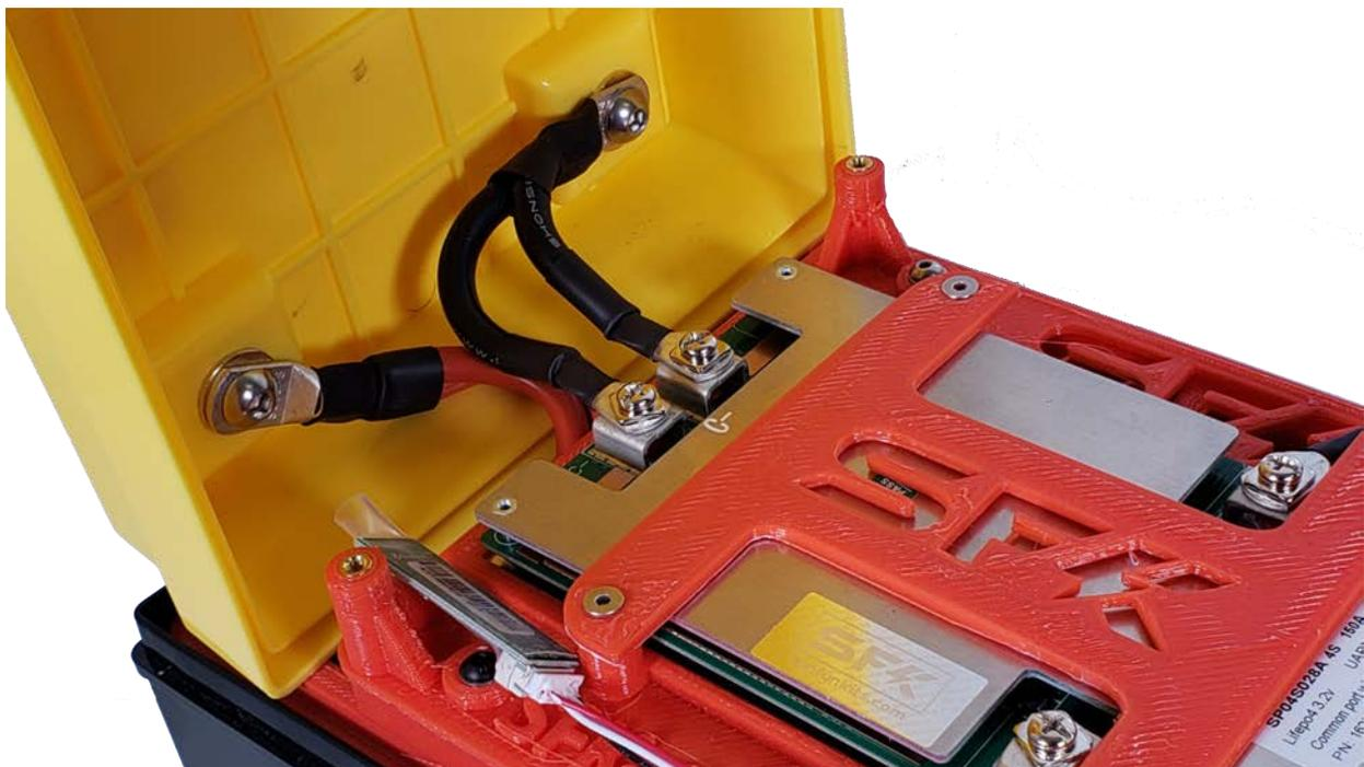
**ENSURE A TIGHT FIT!** You must make sure the bolt is making proper and solid contact to the brass insert, a loose contact will generate heat and can lead to battery failure. Ensure at least 10-15 NM torque setting (appx 140 inch/lbs).
