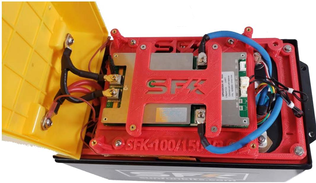
Once the lid wires are secured, you can now insert the balancing wires into your BMS.
