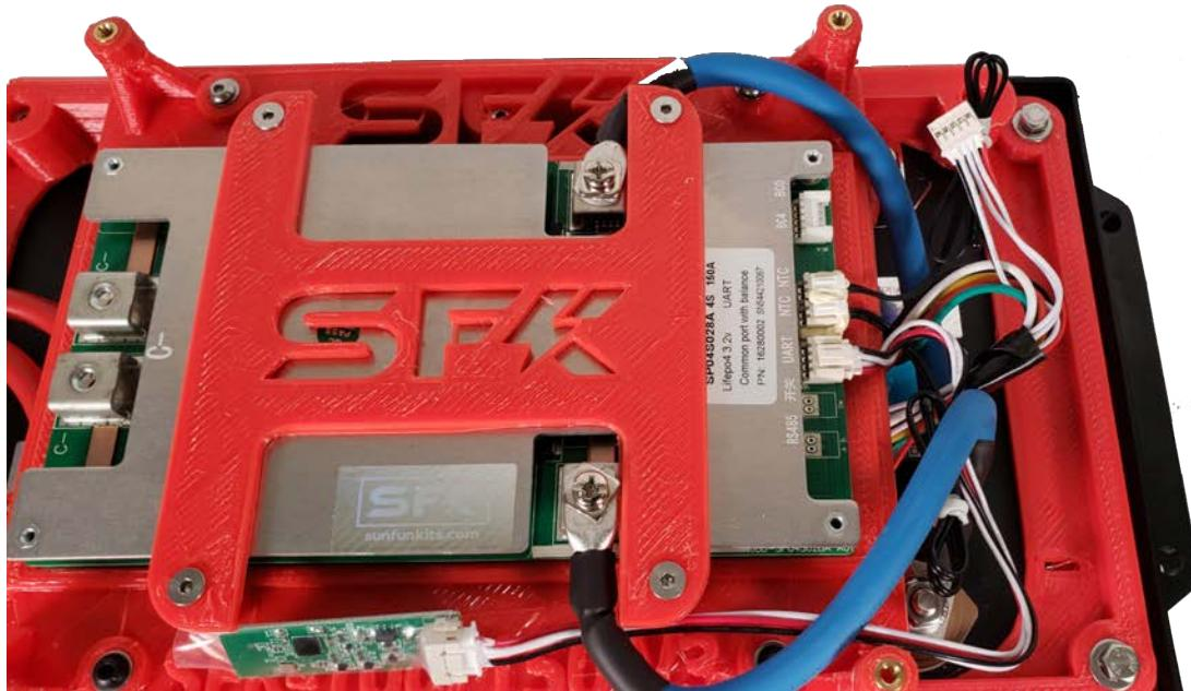
**NOTE:** Make sure the balancing lead is **NOT** connected to the BMS! This will be inserted in a later step.
