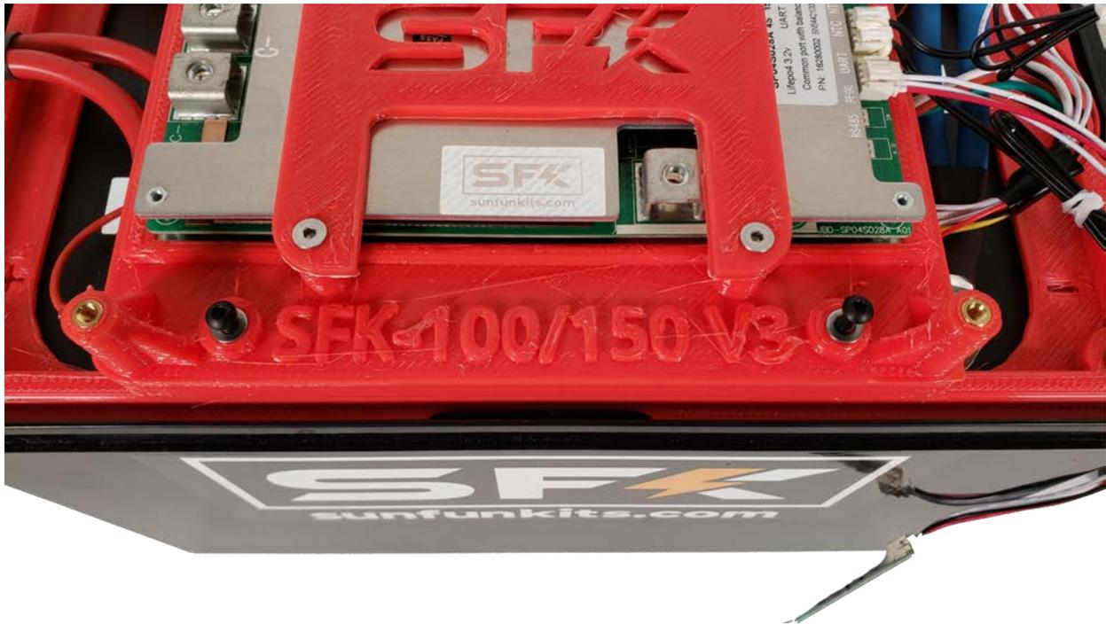
Install the m4x25-30 mm bolts on the bottom, and the m4x15mm bolts on the top.
