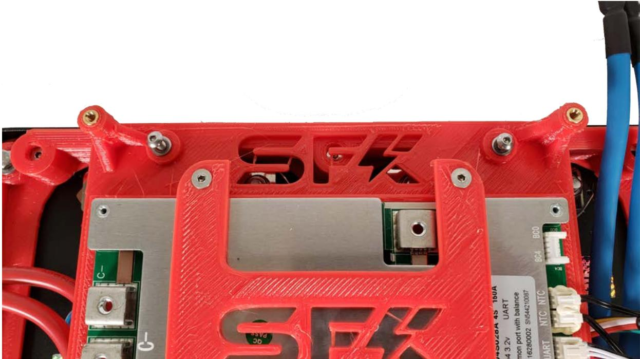
With the plate secured, it is now time to start attaching the terminal cables to the BMS, this will vary depending on which BMS you are using, for all Sun Fun Kits BMS, we provide the BMS to you with appropriately sized crimped and ready-to-install wires that you easily attach to your kit.
