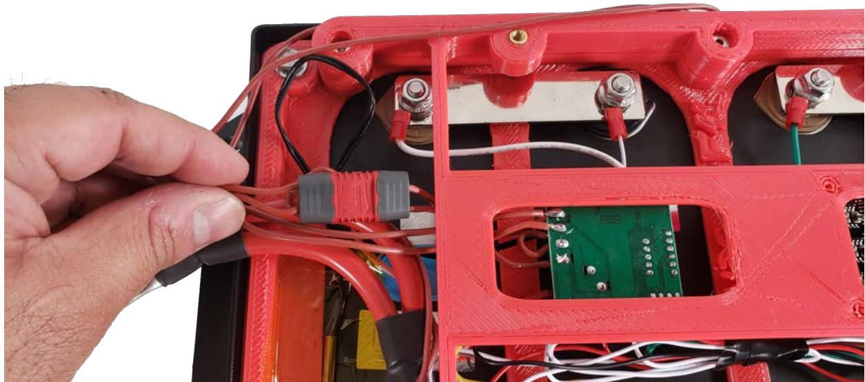
For heated kits you will connect the T-plug to the thermal switch feed to provide the heating elements with power. Tuck under the riser plate and secure it using zip ties, velcro strips, or electrical tape.
