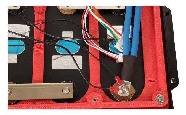
NOTE: be sure to use the included washers for the BMS and Active balancer terminals. This is needed as many cells include serrated nuts that "dig" into the metal, the material on the balancing and active balancing rings may not be sufficient to handle this, hence a washer above and below the terminal is recommended.
