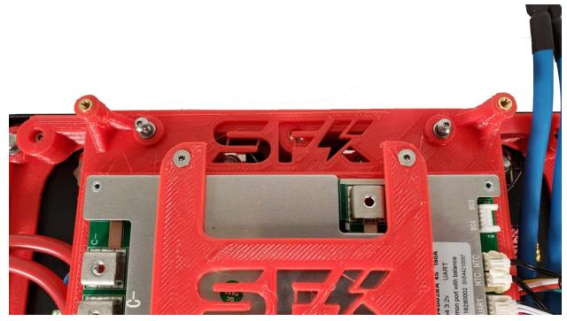
With the plate secured, it is now time to start attaching the terminal cables to the BMS, this will vary depending on which BMS you are using, for all Sun Fun Kits BMS, we provide the BMS to you with appropriately sized crimped and ready-to-install wires that you easily attach to your kit.
