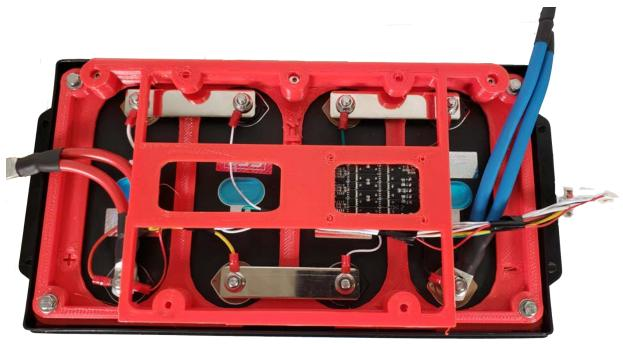
Secure the riser plate using the 3 countersunk M4 screws. We recommend only using hand tools for this process (despite the youtube videos where the installer and author of this manual uses an impact hammer...  $\bigcirc$  ).
