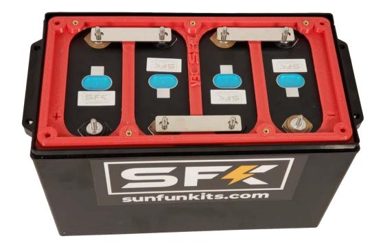
Now you will add your series terminals and BMS balancing/monitoring wires as well as the active balancer wires (NOTE the initial negative post; and the final positive post are shared between both the active balancer & BMS, all other posts may be separate for each cell):
