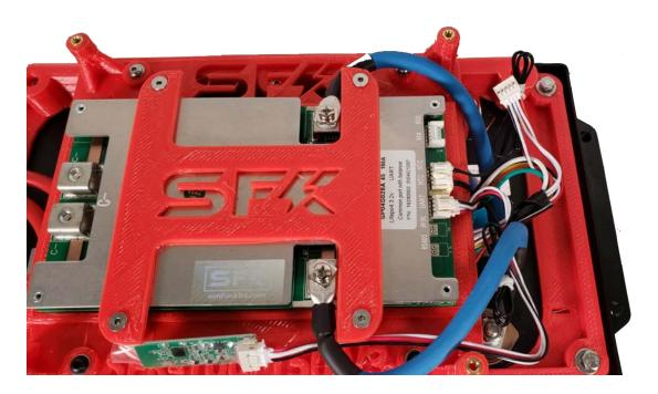
**NOTE:** Make sure the balancing lead is **NOT** connected to the BMS! This will be inserted in a later step.
