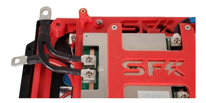
Most BMS units will include one or more NTP probes, these can be mounted at the position of your choice. For The SFK-150V2 BMS unit, you may place these on one of the cells and on a mounting plate (to get internal case temperature).
