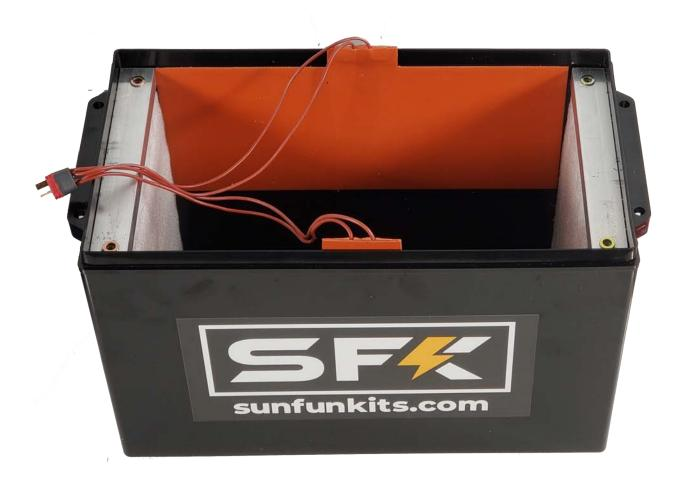
The heated kits will provide additional resistance to cells when they are being installed, however, there is still sufficient space to insert the cells. It is recommended that you do not install fully charged cells as they will make the process challenging.
