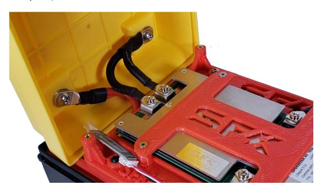
**ENSURE A TIGHT FIT!** You must make sure the bolt is making proper and solid contact to the brass insert, a loose contact will generate heat and can lead to battery failure. Ensure at least 10-15 NM torque setting (appx 140 inch/lbs).
