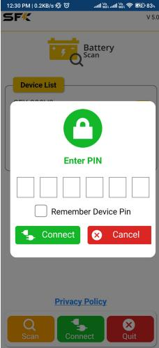
After you have downloaded the app, you will need to enable location services to allow a connection to your SKF-300HP battery. Once enabled you can scan for available devices and connect to the battery you wish. With version 4.X and higher; the SFK BMS app supports up to 4 simultaneous device connections, this is explained on page: 39.
