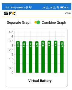
When connected to Multi-View you will notice various options that differ from the single view. Here you can analyze information that represents all of your connected batteries as a single bank. The details tab will display information for your cell voltages per pack, or you can view them together in a single large graph. This is useful to ensure all of your cells are balanced and are working properly as well as able to hold voltage under load.
