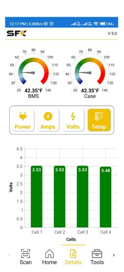
The details tab provides additional information for your battery, this can be useful in finding out issues you may be experiencing such as HVC or LVC (high/low voltage cut-off). If you are finding your cells are being stressed under loads you can use the information to make changes to the load accordingly. NOTE: The SFK-300HP has 3 temperature probes which includes 1BMS probe and 2 case probes, you can switch between the case probe temps by clicking the case temp gauge to switch between them.
