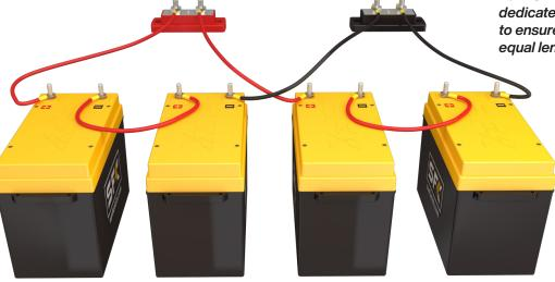
For 2S2P setups, consider the use of dedicated bus bars, you will also need to ensure your parallel cables are of equal length and wire gauge.
