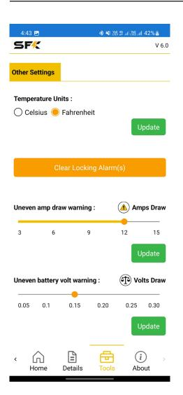
It is important to ensure your batteries are properly balanced before setting up the maximum and minimum SOC limits. Imbalanced batteries can cause this functionality to not work as intended; if your SOC is not properly calibrated per battery, it will cause the app to send incorrect commands to the battery.
