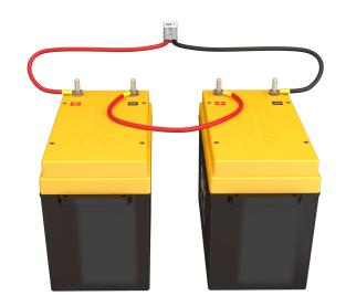
Cables of equal length are recommended but not critical in series setups. We recommend using 2 AWG or lower gauge for best performance.
