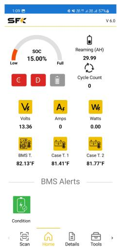
After downloading and connecting to your battery you can view information in 5 tabs. The Main tab will display general battery information like the state of charge of the battery, the temperature, remaining capacity, as well as the current and watt output.
