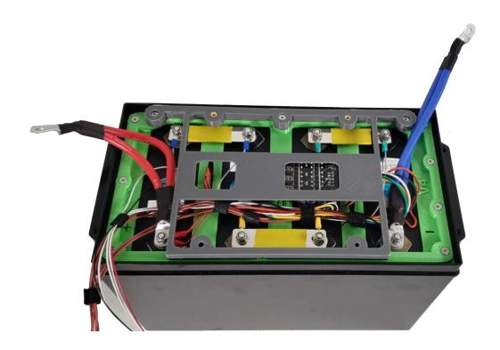
For sidewall heating installs, you will need to secure the heating pad flap to the riser using kapton tape. This is required to ensure that the heating pads do not interfere with the tongue and groove construction of the case and lid.
