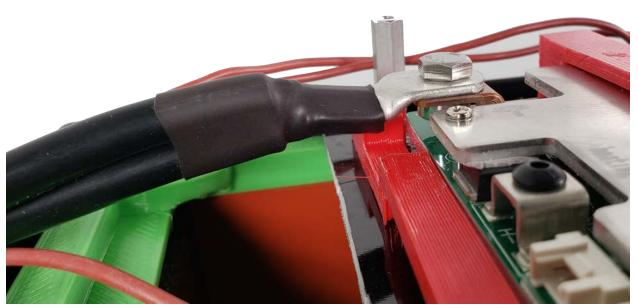
\*Similar to the blue wire, the black bms to case wire is also installed inverted, this allows for greater flexibility in wire routing. Secure with the included M6 hex bolt.
