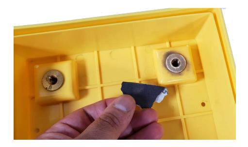
Once cleaned, use isopropyl alcohol to wipe clean and then begin to attach the main BMS and cell wires.
