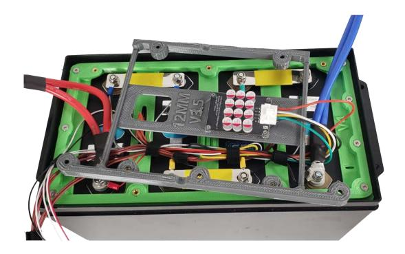
Secure the riser plate using the 3 countersunk M4 screws. We recommend only using hand tools for this process (despite the youtube videos where the installer and author of this manual uses an impact hammer... (2).
