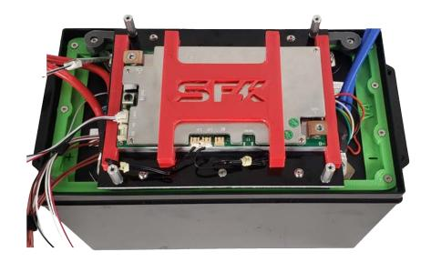
Install the 3x m4-25 mm bolts on the bottom, and the 2x m4-16mm bolts on top of the bms plate. The next step is to prepare the case lid. **NOTE:** Make sure the balancing lead is **NOT** connected to the BMS! This will be inserted in a later step.
