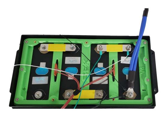
You will align the balancing wires towards the main lugs leaving the center area clear for the active balancer.
