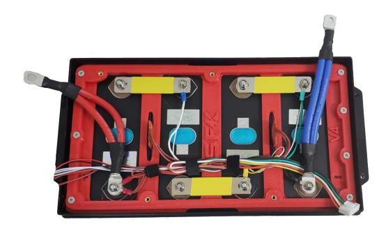
NOTE: The heating pad now shares the main positive of cell 4 and no longer requires a connection to the LID.
