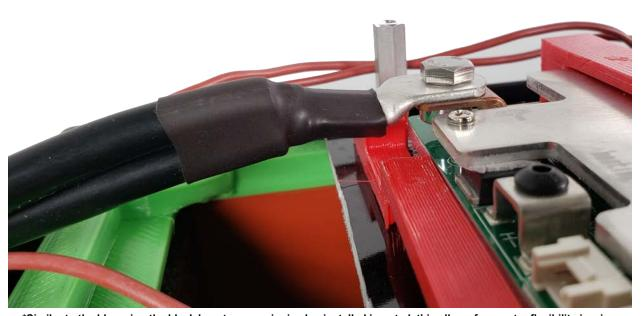
\*Similar to the blue wire, the black bms to case wire is also installed inverted, this allows for greater flexibility in wire routing. Secure with the included M6 hex bolt.
