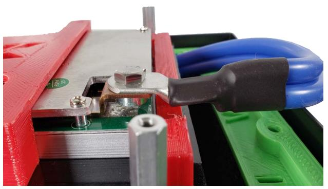
\*The blue wire end with its wires crimped vertically is attached in this inverted lug manor. Secure the wire to the BMS terminal with the included m6 hex bolt.
