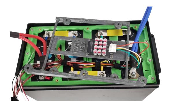
Secure the riser plate using the 3 countersunk M4 screws. We recommend only using hand tools for this process (despite the youtube videos where the installer and author of this manual uses an impact hammer... ).
