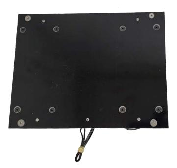
With version 4, we are now using a 3mm / 1/8" thick Garolite FR4 / fiberglass main plate along with aluminum standoffs with custom 3d printed holders to secure the BMS in place. This provides us with superior heat resistance, increased strength, and greater dimensional accuracy for our kits. Many of these changes are in response to queries and suggestions form our
