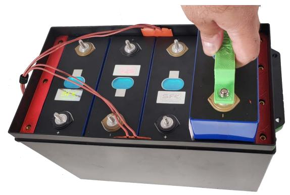
\*Take note of the 1.5mm Shims, these are needed to ensure a level surface for the main cell plate.
