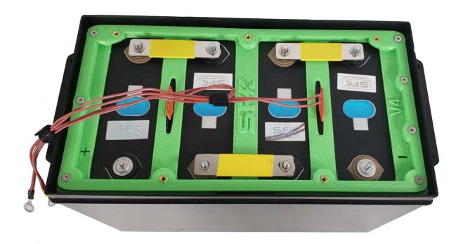
Now you will add your series terminals and BMS balancing/monitoring wires as well as the active balancer wires (NOTE the initial negative post; and the final positive post are shared between both the active balancer & BMS, all other posts may be separate for each cell). Place the BMS ring terminal directly over the main lug and then the active balancer ring on top of it.
