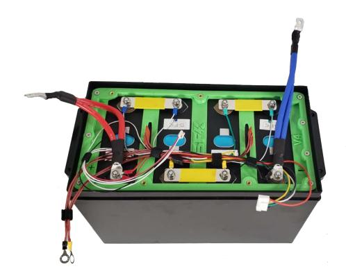
USE EXTREME CAUTION! THE BLUE WIRE SHOULD NOT TOUCH THE POSITIVE TERMINAL OF THE FIRST CELL OR IT WILL ARC AND DESTROY THE CELL. You should consider covering this terminal with kapton tape or other insulating material to ensure that it can not short circuit the first cell.
